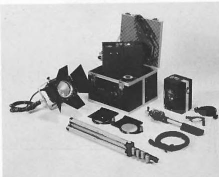
watts) of the open face type which gives both spot and flood facility. HMI lights have requirements for stringent safety regulations all of which are adequately met with the Colortran UK units. Micro switches engineered into the flanges are held into position by the safety glass. Should a glass break, the micro switch pops out of its seating to break the circuit and instantly switch off the supply to the lamp. These and other features make this lamp safe in all applications.
