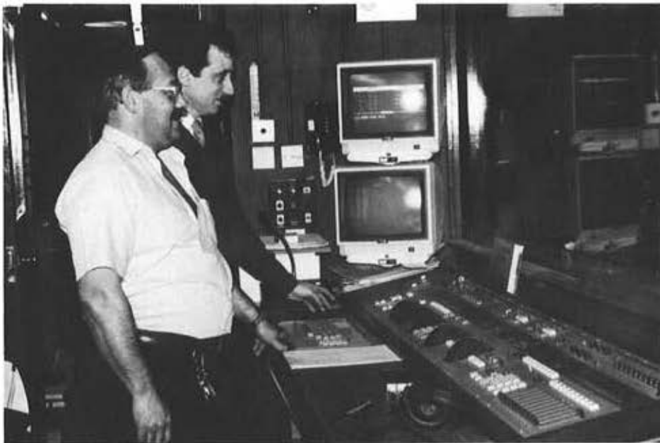
Andy Kent, the Theatre Royal's chief electrician, pictured with Northern Light's Jonathan Allen in the FOH lighting control room. The board is a Strand Galaxy 2 Premier.
