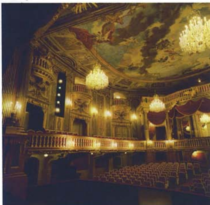
The majestic Schönbrunner Schlosstheater at the Schönbrunn Palace, Vienna. Ludwig Pani installed motorised shutters for the front of house lighting so that the units are hidden when the theatre is not used for a performance.
