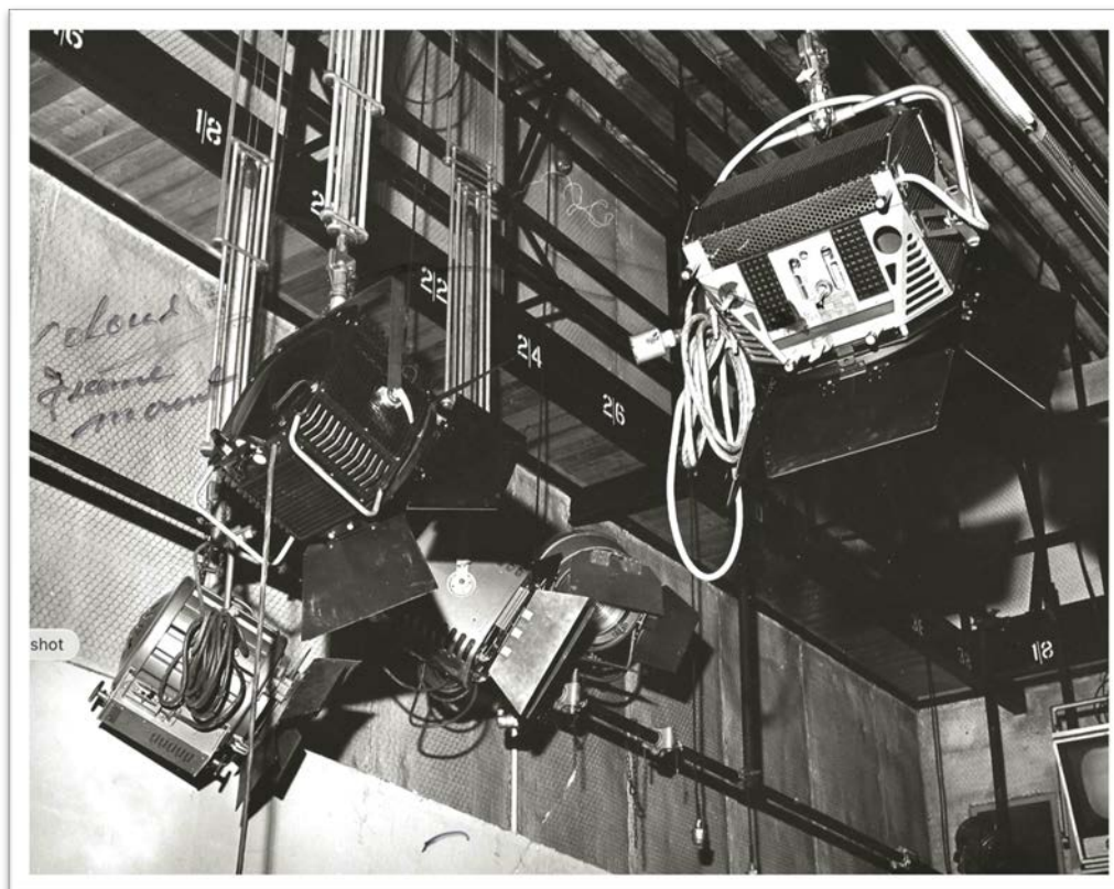
Figure 3. Prototype Patt. 543 5kW Fresnel undergoing comparative studio testing within a BBC environment alongside competing luminaires. The proposed production model was ultimately not released following Rank's agreement to market Quartzcolor products. Photograph courtesy of Alan Luxford
