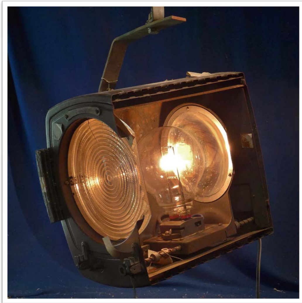
Figure 1. Strand Patt. 243 cutaway lantern showing the internal optical arrangement, including the 10-inch Fresnel lens, lamp, reflector, and focusing assembly. This surviving demonstration cutaway formed part of Strand Electric's showroom display heritage. HSLC Collection.
