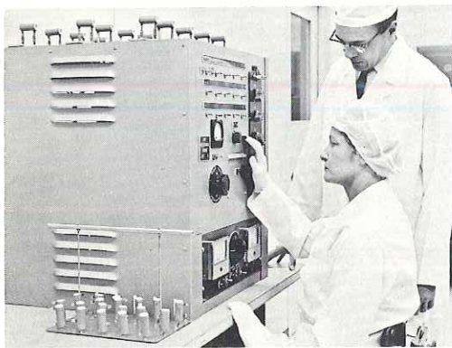
White room within the Mount Vernon plant is air-conditioned, humidity controlled, dust-free and dirt-free and is designed for producing high reliability power resistors. Photo above shows oceanic telephone cable resistors undergoing test on a hot resistance bridge designed and built by Ward Leonard.
