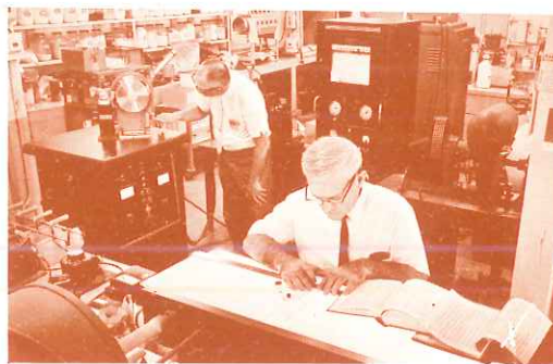
The Mount Vernon R & D laboratory employs sophisticated equipment in development, investigation and quality control of electrical-electronic components. Photo above shows the x-ray diffractometer being used by research scientists for analyzing component materials.
