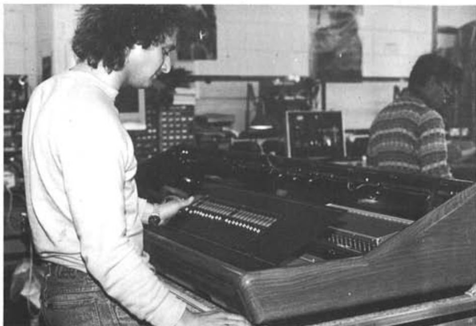
Mark Thompson, service engineer, pictured alongside a QM chassis and matrix panel.
