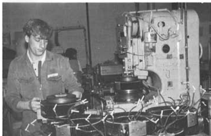
Wiring rheostats - a long ADB tradition.
