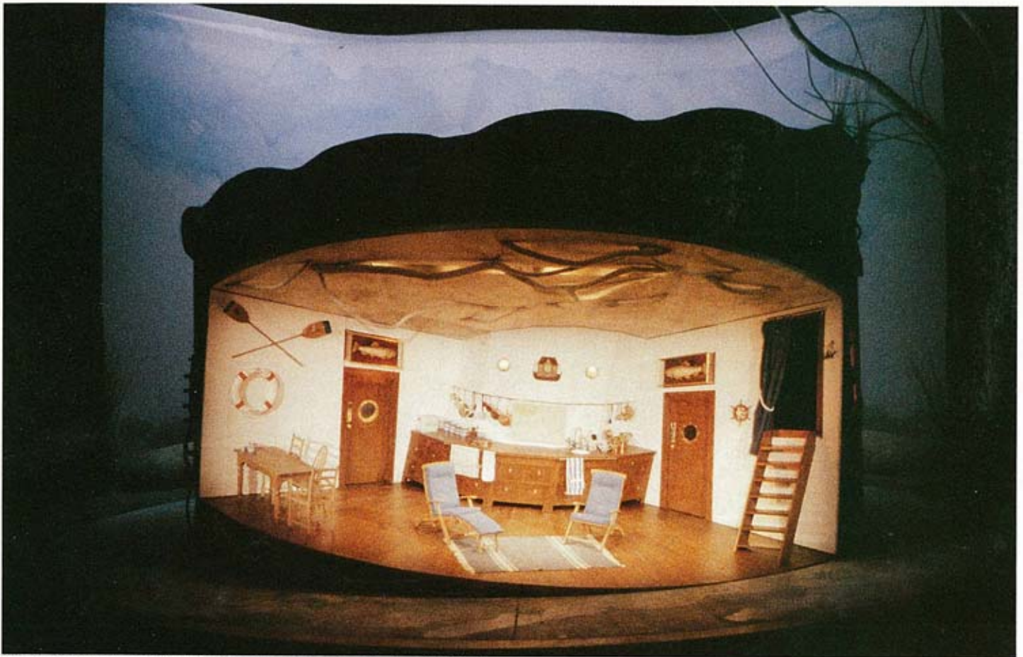
The rotating and rising drum revolve stage showing the interior of Ratty's House.
