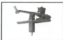
'Sky hook' adjustable gaffer grip with 16mm socket on jaw and 16mm spigot on handle (jaws adjustable from 25mm to 65mm) 53 043 09
