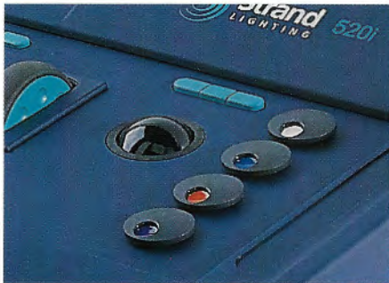
Motion control is fully integrated into all 500 series consoles with a dedicated trackball and rotary encoders to access moving light attributes
