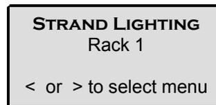
When the self-tests are complete the PROCESSOR OK LED on the front of the processor module will turn ON, and the default text will show on the LCD display.
