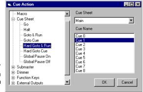
Choose your "Button Down Action" and "Button Up Action" here. You can activate a Macro, run a cue, activate a Submaster, change a dimmer property, activate a Function Key, or activate external outputs.
