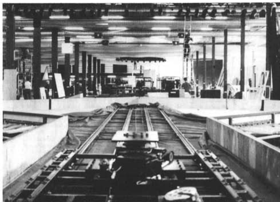
Looking from upstage centre to downstage centre, showing tracking revolve in the tank.
